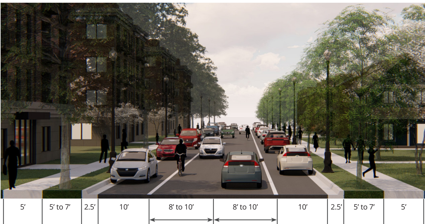
Figure 5.9 (1) Typical Plan and Section for Neighborhood Street Type.
