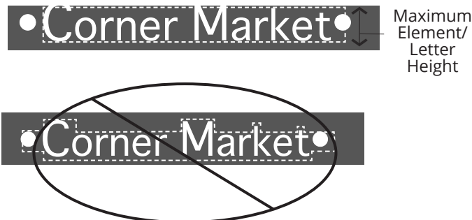
Figure 10.3 (1). Measuring Wall Signs.
